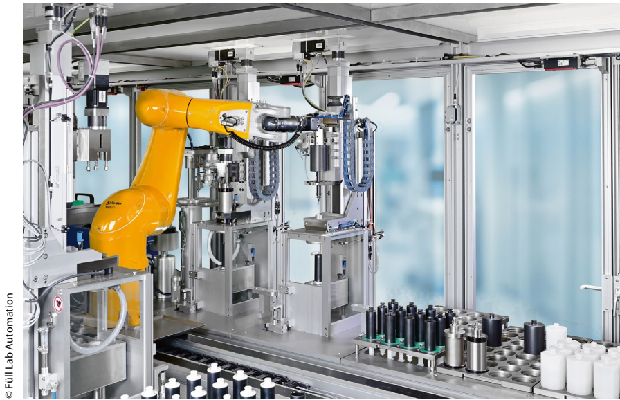
Figure 5 > The handling robot transports a raw material syringe.
